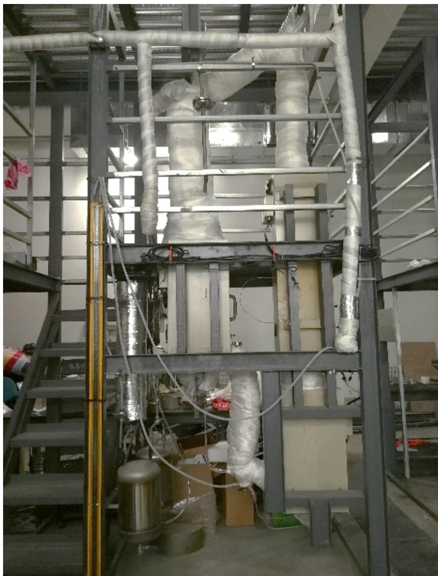
**Fig. 1** . Schematic diagram of a circulating fluidized bed scaled-up reactor.
