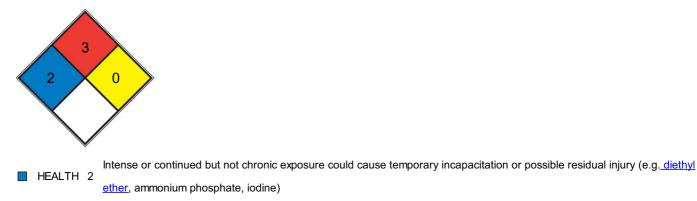
Liquids and solids (including finely divided suspended solids) that can be ignited under almost all ambient temperature
