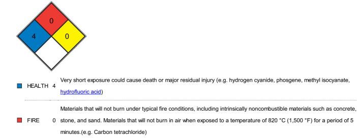
0 Normally stable, even under fire exposure conditions, and is not reactive with water (e.g. helium, N2)
