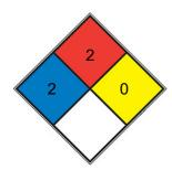
Intense or continued but not chronic exposure could cause temporary incapacitation or possible residual injury (e.g. diethylether, ammonium phosphate, iodine)
