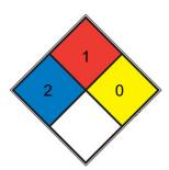
Materials that require considerable preheating, under all ambient temperature conditions, before ignition and combustion
