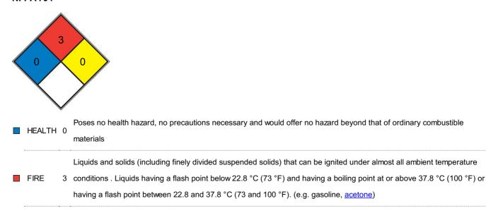
REACT 0 Normally stable, even under fire exposure conditions, and is not reactive with water (e.g. helium, N2)
