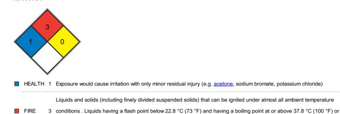
REACT 0 Normally stable, even under fire exposure conditions, and is not reactive with water (e.g. helium, N2)
